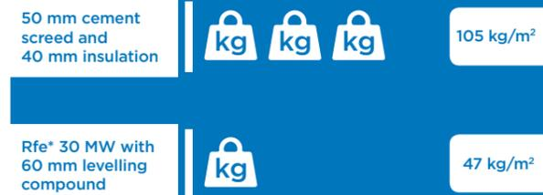
Weigh up a further advantage of dry screed: **\*Rigidur flooring elements** weigh less than half as much as cement screed of the same height. This significantly lower ceiling load goes hand in hand with greater flexibility in designing your floor.
