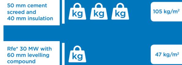
Weigh up a further advantage of dry screed: **\*Rigidur flooring elements** weigh less than half as much as cement screed of the same height. This significantly lower ceiling load goes hand in hand with greater flexibility in designing your floor.
