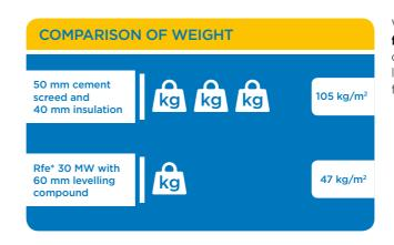
Weigh up a further advantage of dry screed: \*Rigidur flooring elements weigh less than half as much as cement screed of the same height. This significantly lower ceiling load goes hand in hand with greater flexibility in designing your floor.
