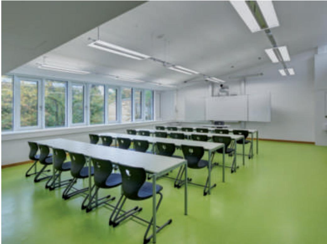
The lighting of the main building is supplied by LED light technology. One differentiates between areas with high-quality lighting tied to a workplace and generally lighted areas. The amount of lightness is regulated by LED luminaires controlled by daylight and presence.
