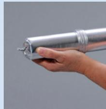
Insert the bag containing the Rigitone Mix into the pistol and cut off the seal.
